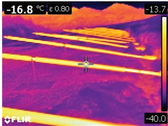
Figure 4: Thermal image of temporary radiators showing temperature gradient between functioning thermosyphon radiators (yellow) and ambient background (red-purple)
