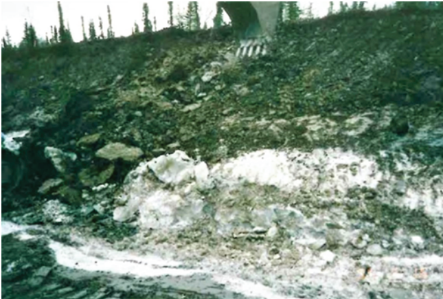
Figure 1: Massive ground ice identified at Dry Creek in 1994/1995 (photo by Government of Yukon)
